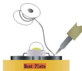
**Use Soldering Iron to solder the leads of Emitter within 5 seconds**
