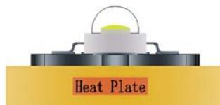
Put MCPCB on Heat Plate until Solder Paste melt. Put Emitter on MCPCB. Take the MCPCB out
